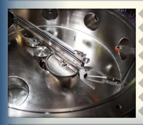
Substrate storage chamber - up to 6 samples
