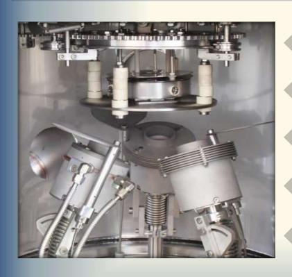
Substrate IR heating up to 400° C
